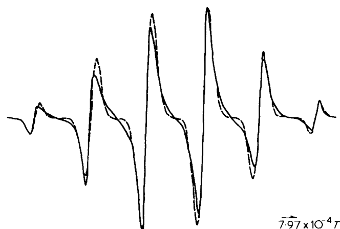
Figure 11 Comparison of the experimental e.s.r. spectrum of alkyl radicals observed at 254K with calculated spectra. \delta = 0^\circ . — — —, Experimental; —, calculated, \Delta H_{\beta 1} = 30.2 \times 10^{-4} \text{ T} , \Delta H_{\beta 2} = 33.8 \times 10^{-4} \text{ T}
